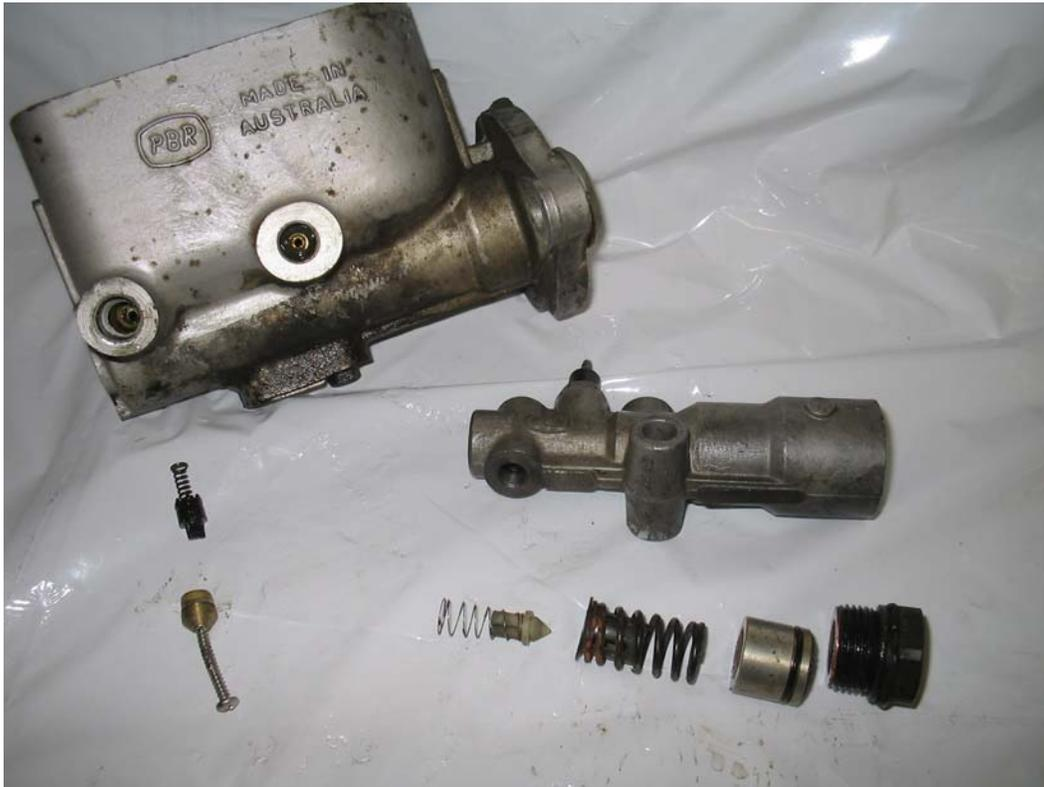
HK -HZ or Torana Master cylinder, check for residual valve by probing with paperclip, pull brass seat with self tapper. Discard valve when using discs on this system.
