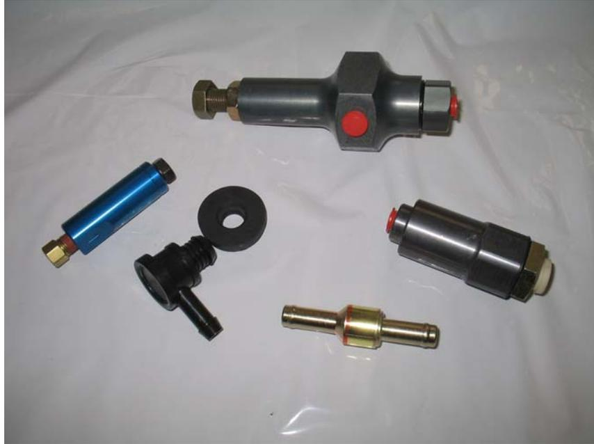
Adjustable Proportioning valve at top, fixed setting 150psi HQ prop valve on right, 2psi in line residual valve on Left, Booster fitted one way vacuum valve on lower left, inline vacuum valve on lower right.
