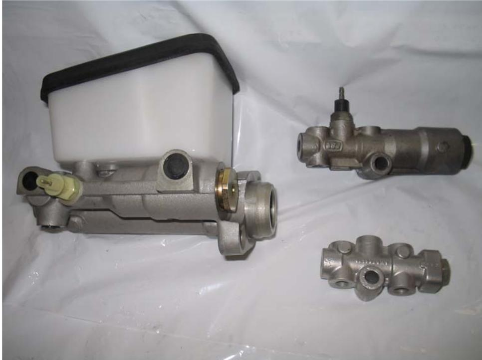
Late type PBR master cylinder with combined proportioning valve and brake fail switch on left.
