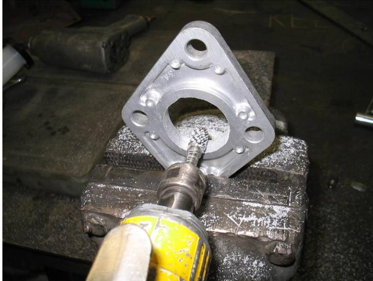
4/ Screw the adjuster bolt on the booster outlet shaft all the way in. Refit the alloy spacer block. It is easier if you remove the pushrod from the booster but be careful not to lose the reaction disc. This should set the pushrod so that it just touches the master cylinder as they are bolted home.
