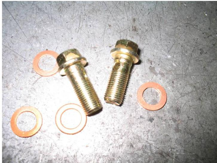
6/One banjo bolt may need shortening so that it properly compresses the copper washers and does not bottom out.
