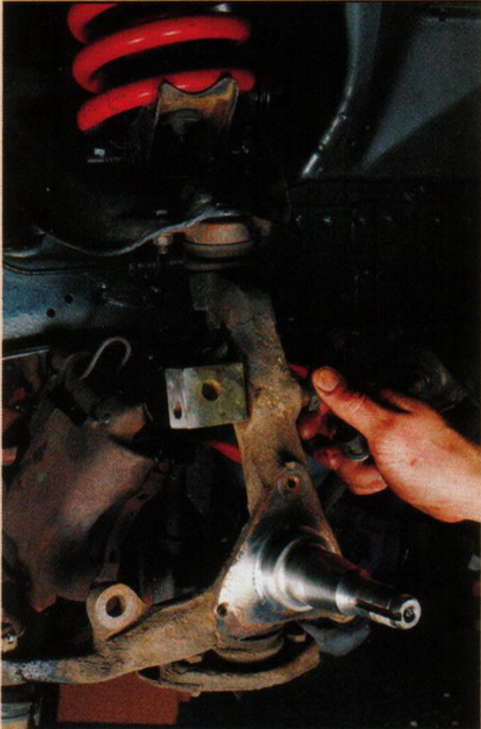
Above: The kit contains a steel block with two holes, each of which runs at 90° to the other. It's fitted to the top bolt hole as shown and becomes the top fixing point for the caliper adaptor plate. This block should be left fairly loose until the other components have been fitted.
