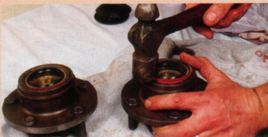
Below: Your new seals have to be tapped into place as shown. Tap evenly right around the edge and be fairly gentle to avoid damaging the seal. Put a little grease on the inside of the seal to avoid having it run dry on the stub-axle.
