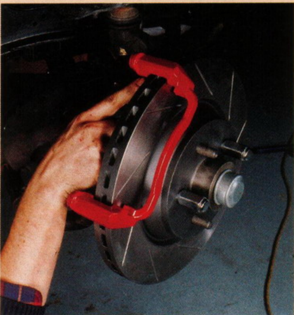
Above: The disc is fitted over the hub and is held in place with a couple of wheel nuts.
