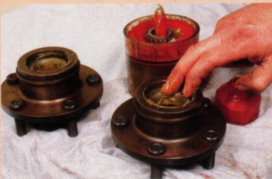
Below: Your new seals have to be tapped into place as shown. Tap evenly right around the edge and be fairly gentle to avoid damaging the seal. Put a little grease on the inside of the seal to avoid having it run dry on the stub-axle.
