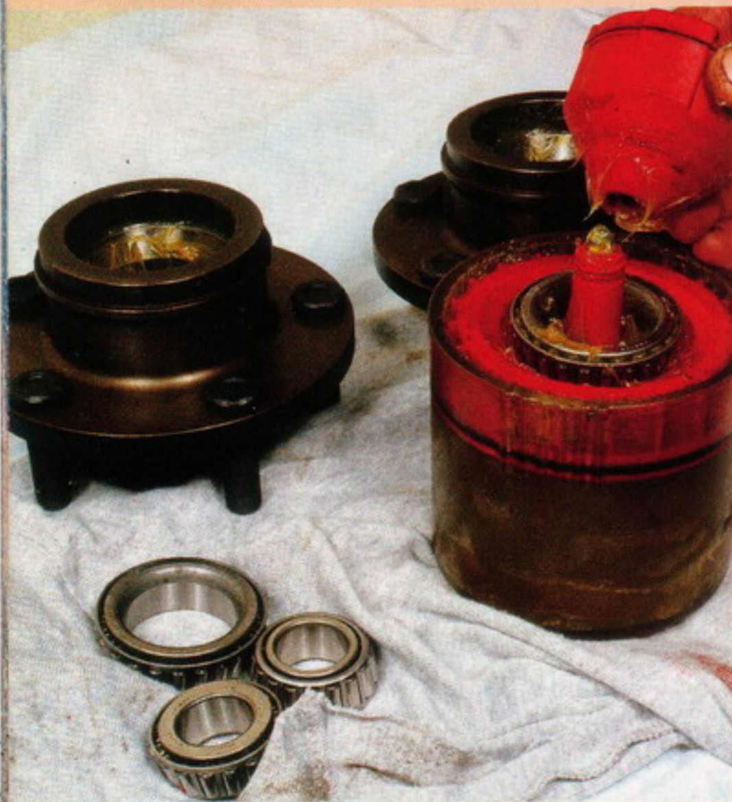
Above: Bearings need grease. Traditionally, you simply take hold of it, grab a handful of bearing grease and start pushing it through the rollers. One of these handy little grease container/bearing packers makes things much easier if you have, or can borrow, one.
